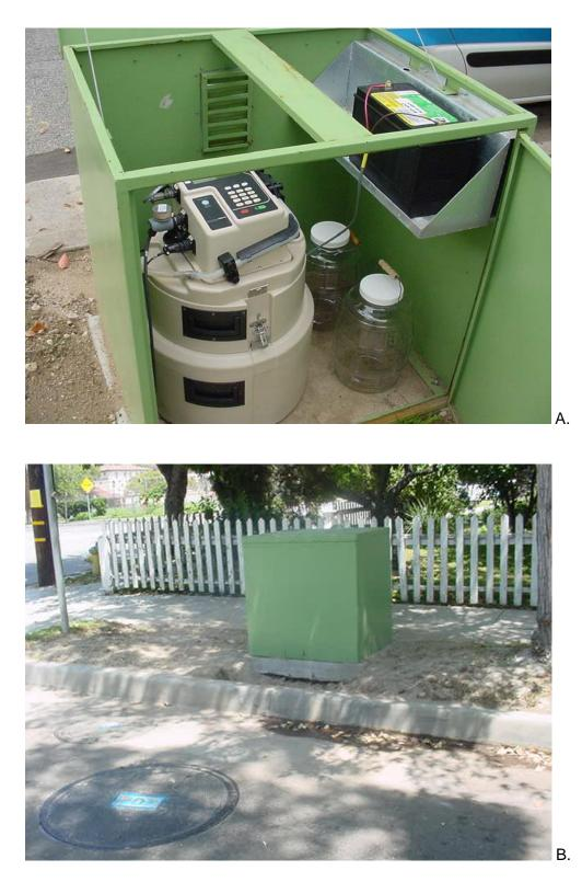
**Figure 8.** A. Autosampler contained within green housing box at the South Pasadena site. B. Housing containing the autosampler located next to the manhole cover of the CDS unit.
