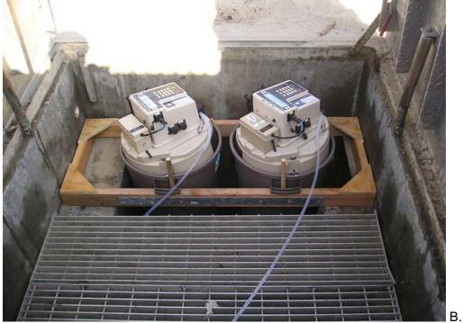
**Figure 6.** A. CDS unit at the Pico-Kenter site. B. Influent and effluent autosamplers in a pit adjacent to the Pico-Kenter CDS unit.
